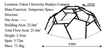
Figure 7: Determination of the shape of the dome
