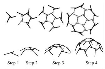
Figure 13: Determining the shape of this dome, which creates a space by overlapping members
