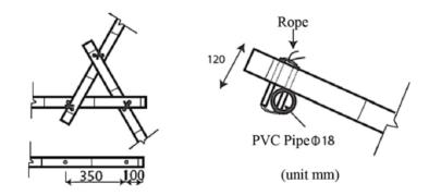
Figure 10: Detailed view of the joint used for this dome
