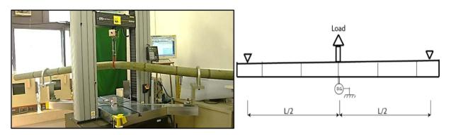
Figure 3: Three-point Bending Experiment
