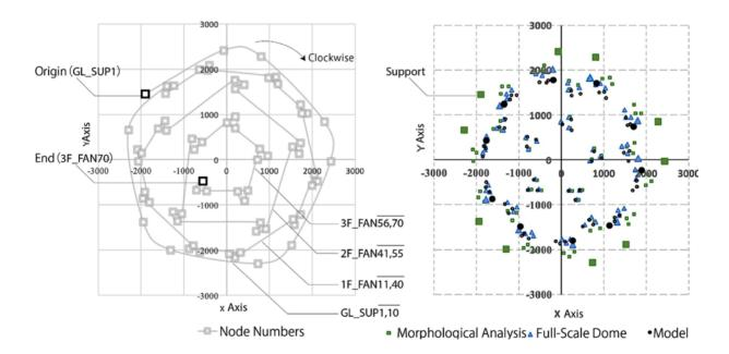
Figure 8: Comparison of Coordinates from the Top view
