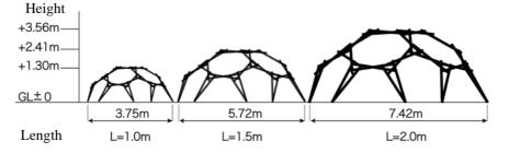
Figure 6: Relationship between member length and dome height
