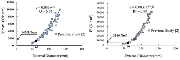
Figure 4: Relationship between  $M_{max}$ , EI and the external diameter, respectively.
