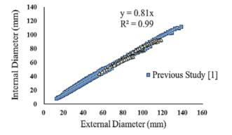
Figure 2: Relationship between internal and external diameter
